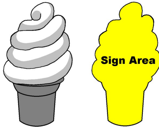
Figure 3.10E – Area of a Three-Dimensional Sign
