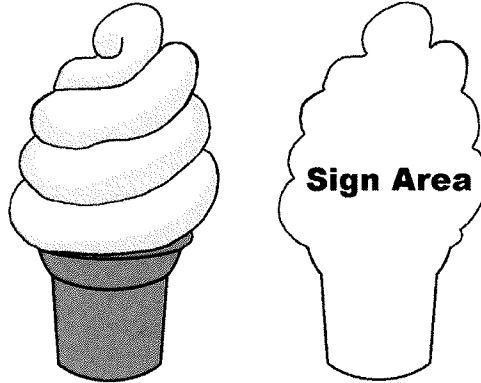
Figure 3.110E – Area of a Three-Dimensional Sign
