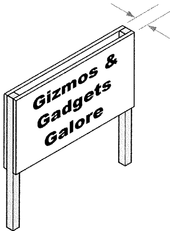
Figure 3.110C – Sign Faces Less than 30 Degrees Apart
