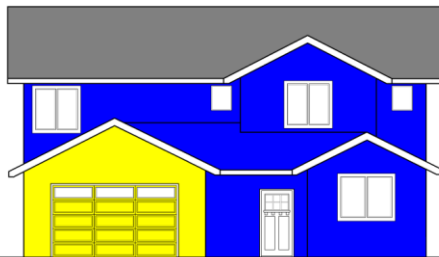
Figure 3.107A – Garage (yellow) comprises less than half the lateral dimension of the facade (yellow plus blue)
