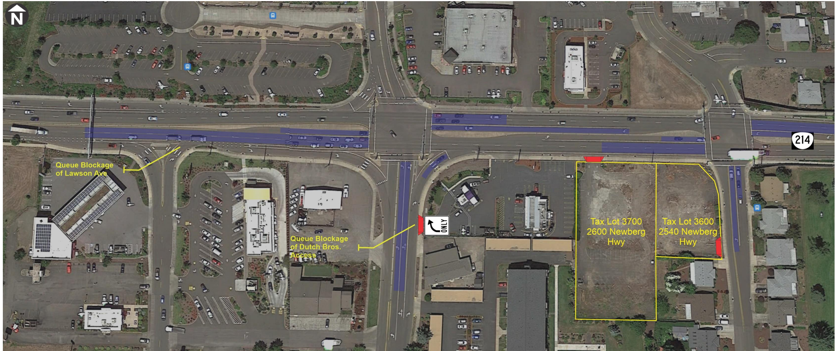
Figure 18. Year 2025 95 th Percentile Queues with Right-In Only access from the Newberg Highway.
