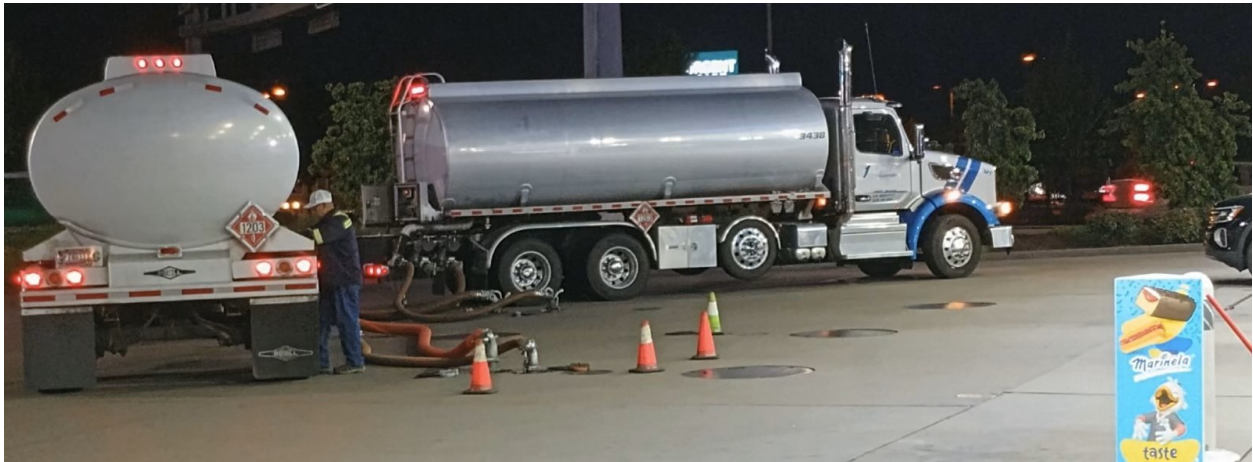
Figure 4. Typical fuel truck offloading process.
