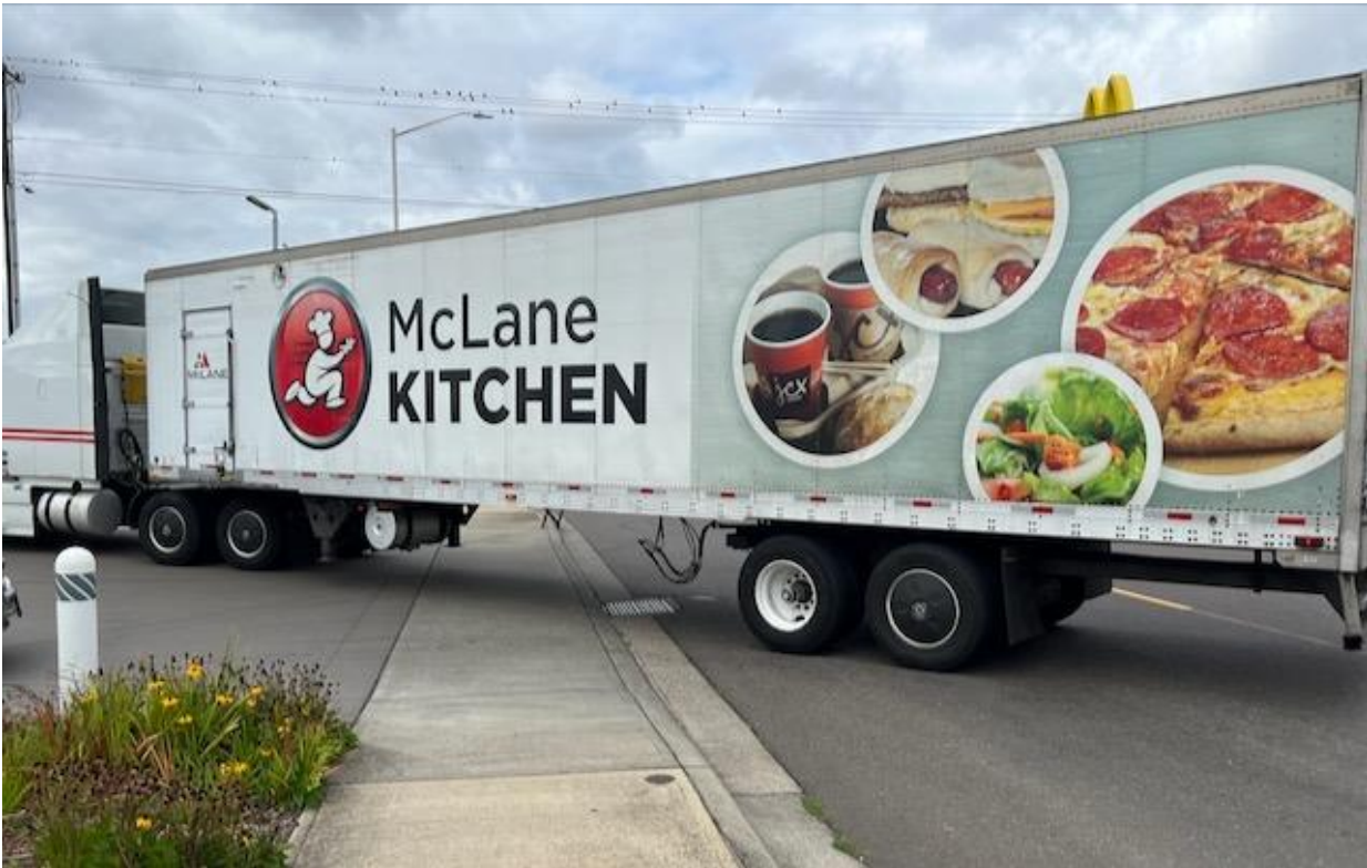
Figure 9. Semi-truck entering the Arco at a shallow angle through the southbound Lawson Avenue travel lane to avoid driving over curbs
