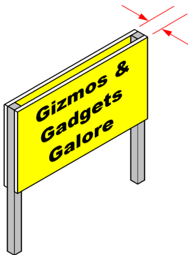
Figure 3.10C – Sign Faces Less than 30 Degrees Apart
