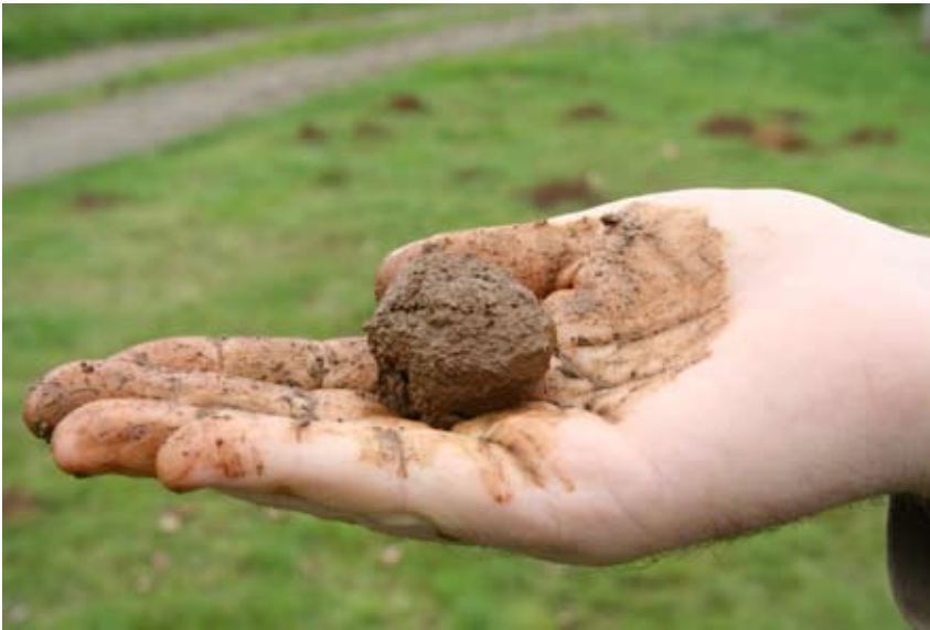
Figure 7a: Conducting a soil feel test by making a ball with the moistened soil, to see how easily it falls apart as well as what texture it has (sticky, silky, or gritty). (Photo: Gina Emanuel)
