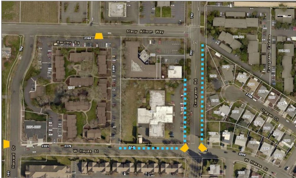
Exhibit T-BP North: This exhibit illustrates locations and represents improvements related to Conditions T-BP1 through 5. Sidewalk is in blue dashes and ADA ramps are in yellow trapezoids.
